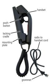
Using private handset mode, the radios internal and external speakers are muted and the call can only be heard from the handset earpiece.
